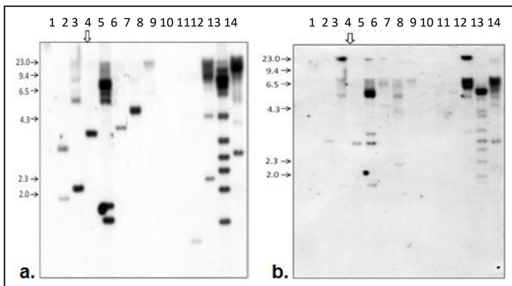
**Figure 4.8:** Southern blot analysis to identify single copy insertion line for the *barstar* construct (designated later as event modbs 2.99). Genomic DNA digested with EcoRV enzyme and (a) Probed with *bar* gene coding sequence present towards the Left border of T-DNA and (b) probed with *barstar* gene coding sequence present towards the Right border. Lane 4 (marked with arrow) represents the selected Event modbs 2.99.
