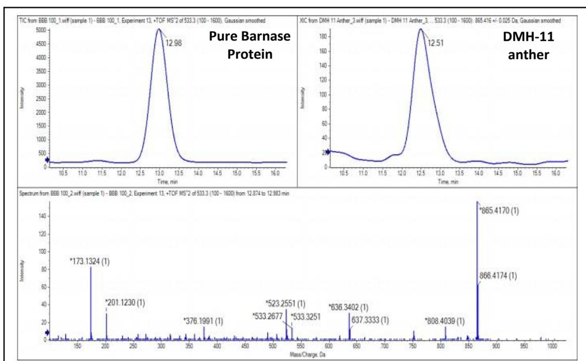
**Figure 4.11:** The extracted ion chromatogram for barnase peptide SIGGDIFSNR from the pure protein and DMH-11 anther. The MS/MS is shown for the pure protein.
